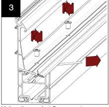
Using the socket flange nuts provided locate them on the bolts. Once all nuts have been located on their corresponding bolts fully peel back the sealing tape film on both sides and tighten down the nuts.
