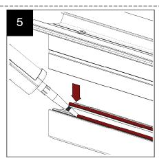
Apply sealant to the frames to ensure a weather tight seal between the bolster and the frames. Once the sealant has been applied lower the bolstered eaves onto the frames
