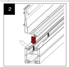
Lift the eaves beam onto the bi fold support beam ensuring the bolt channel is positioned to the inside and taking care to allign the drilled holes with the bolts.
