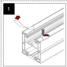
Peel back a small tab of the sealing tape protective film. Ensure the 'tail' is accessable from the side of the bolster.
