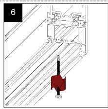
Fix the bolster to the frames using self drilling screws through the frames and up into the bolster. If steel reinforcement is included in the frames it may require predrilling.
