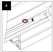
Using sealant apply around the heads of the fixings ensuring a water tight seal.
