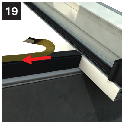
MS Polymer sealant only on Self cleaning glass MS Polymer
