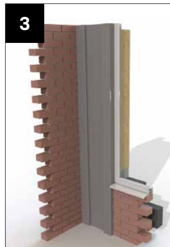
3 Column sat on dwarf wall, claddings run to ground (retro fit situation)
