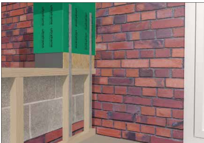
STRAPS MUST LINE UP WITH STUDWORK
