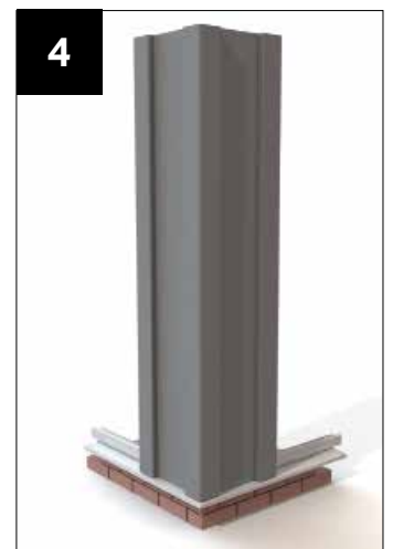
Sat on cill - Column sits on base, external edge of column is notched to allow external cill to run round (see page 17).
