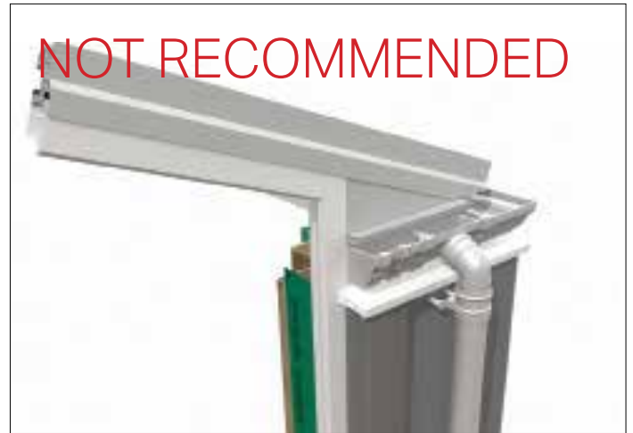
SHORT RETURN WITH CILL. If unable to return back to house wall use inline outlet for 67° obtuse round, positioned centrally on column.
