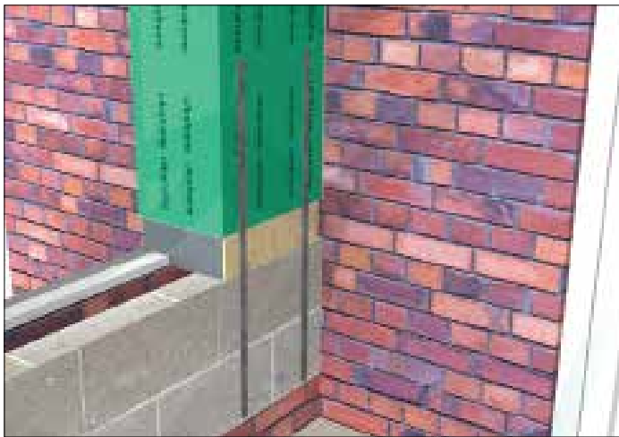
ABUTMENT Fasten straps down inside of wall of abutment column
