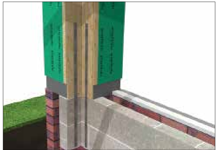
LARGE 90° CORNER Fasten straps down inside of walls of large 90° corner column
