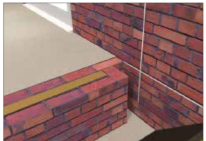
If a concealed rainwater downpipe has been specified on the Abutment column, then the base work is required to step in to allow for the downpipe to exit below the column directly into a drain. Right hand column required here.
