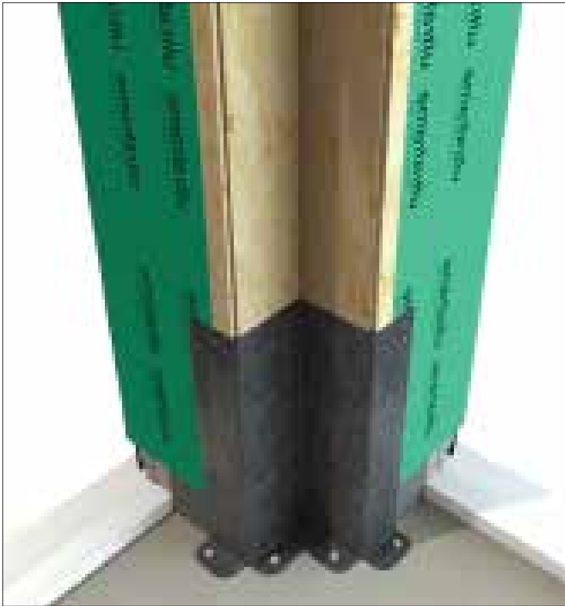
Internal structural steel plate is anchored to slab. Plate may require recessing dependant on finished floor.
