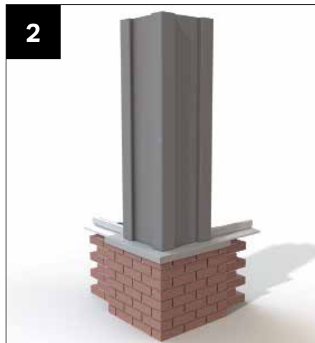
Claddings with masonry Plinth Cap
