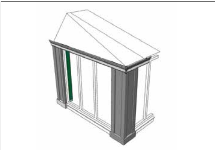
Hipped end with abutment
