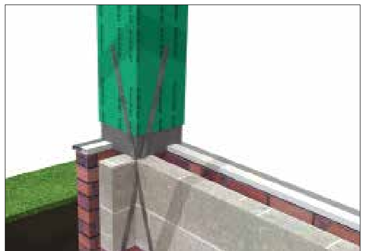
SMALL 90° CORNER Fasten straps down inside of walls of small 90° corner column. Internal brickwork will require grinding to create relief for strps to cross over.
