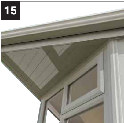
15 Cut and fit ship lap to suit.
