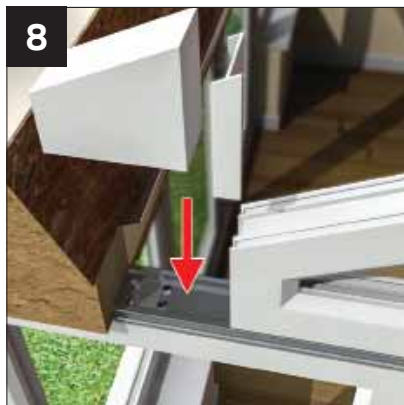
Apply silicone to the gable support extrusion and fix the gable frame. Trial fit the infill wedge and coupler prior to final fixing.
