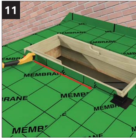
11 Ensure membrane is fitted neatly against the aperture and staple in position and trim.
