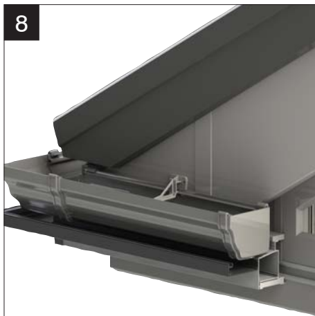
8 Fit the lower Cornice section followed by the guttering. Use face-fix gutter bracket supplied to secure gutter at mid-span of returning gutter as shown.
