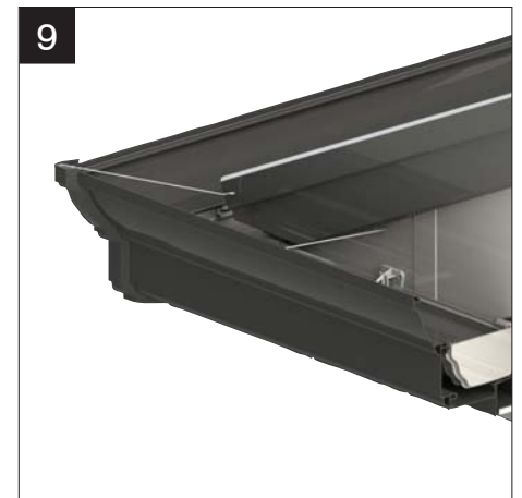
9 Fit remaining cornice components and secure using two tie wires. Fix wires into the barge board face below the top line of the cornice (tie wires may require bending to suit). Fix using self drilling screws CRN010.
