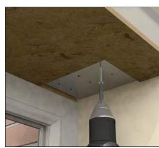
Fixing wall brackets to the beam
