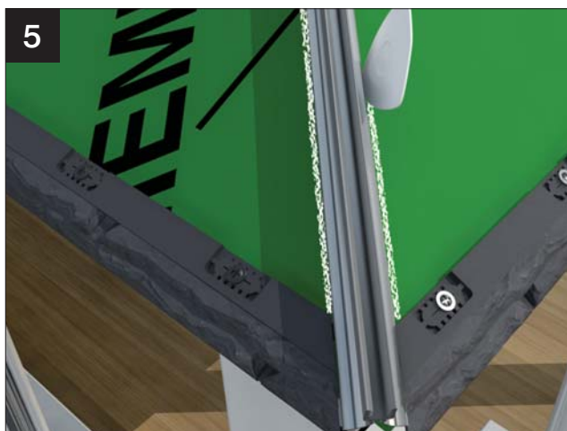
Mark position of hip spines and remove from roof, this helps with fitting of the tile panels.
