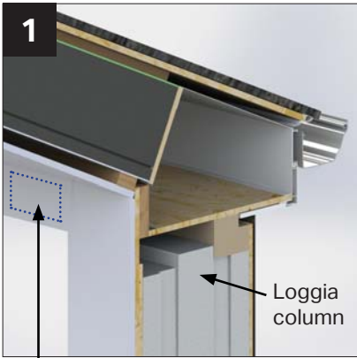
1 Double board adjacent to OSB cladding
