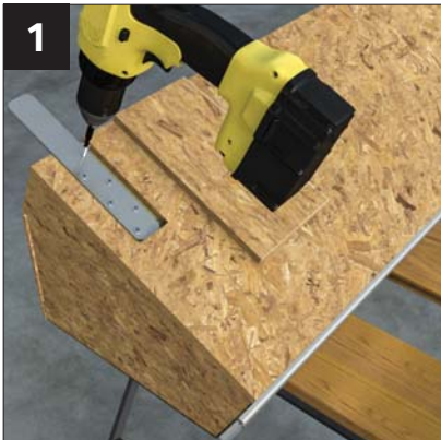
1 Fix the aluminium gable beam fixing plate to the underside of the box beam using 6 x RRR 025 screws. NOTE: ALIGN PLATE 'V' NOTCH GROOVES WITH EDGE OF BEAM.
