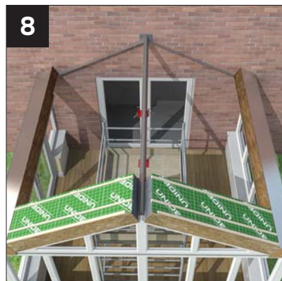
8 Referring to the panel layout sheet, fit the first panels at the gable end as shown in images 35 to 37 on page 23.
