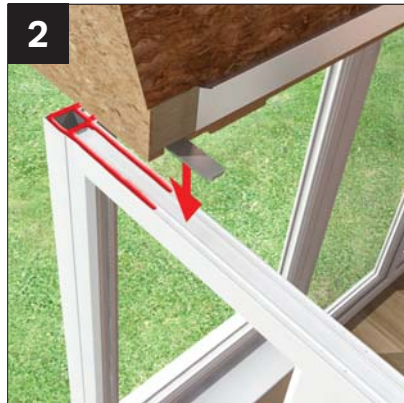
2 Apply low modulus silicone to the head of frames local to beam area before lifting the box beam into position. Temporarily fix the box beam in position.
