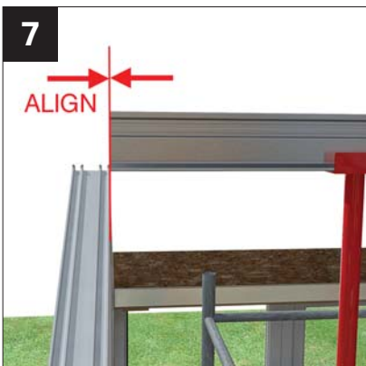
7 After installing the ridge as detailed in pages 22 and 23, images 25 to 30, check that the end of the ridge is in line with the gable end internal frame line.
