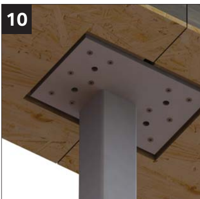
Once both beams are in place, secure the post into the beams. (Fix through the 12 counter sunk holes using the screws provided.)
