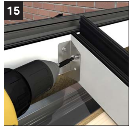
15 Again, check intermediate bar for squareness, then secure with 4 x 4.2mm x 25mm (NRTS 050) provided. Repeat on opposite side
