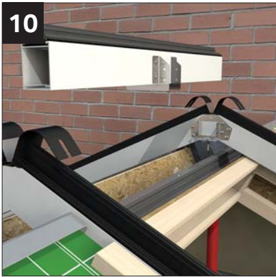
10 Locate the glazing ridge/spacer beam into the adjustable bracket shoes. Check 'A' frames are parallel to each other.
