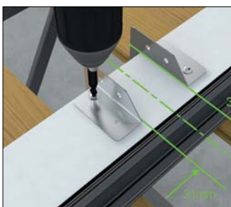
Fixing intermediate glazing bar bracket
