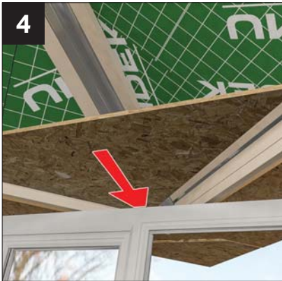
4 Slide into position additional external OSB board.
