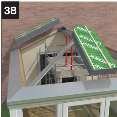
Fit front central panel in-line with ridge.
