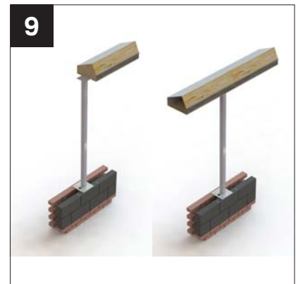
Once secured, place the first box beam onto the post followed by the second beam.
