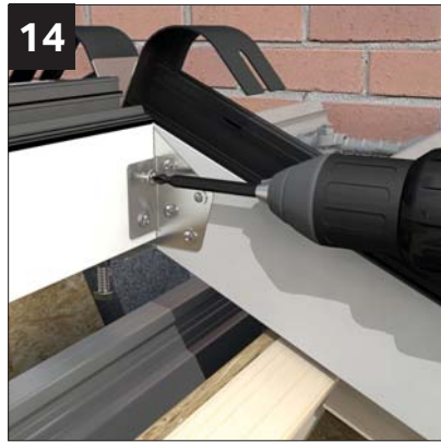
14 Ensure glazing section is square, checking diagonals are equal. Secure adjustable connection bracket into ridge spacer beam using 4 x 4.2mm x 25mm (NRTS 050) provided. Repeat on opposite side of 'A' frame.
