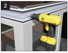
Two pilot holes already exist in the next piece of eaves beam – drill two more at 4.5mm diameter through the eaves beam and the cleat and then securely fit the four M5 x 12mm taptite screws.
