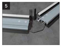
Take the second starter bar and similarly offer this onto the ridge hanger/compression plate assembly. Lift the whole "A" frame assembly and get ready to install it in its final position.
