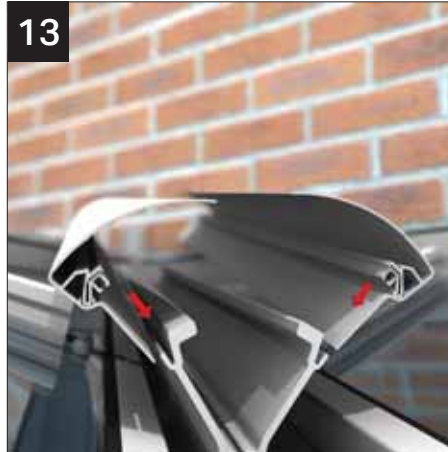
Locate second half of valley cladding over siliconed cladding. Ensure cladding pushed fully down.
