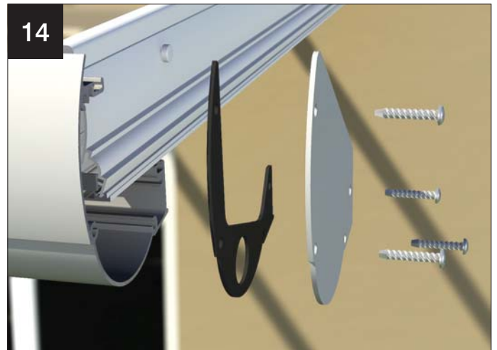
Fit the profiled rubber gasket and end plate to the curved beam using 4 x M8 button head hex screws (AVBA014) provided. Repeat on the opposite side.
