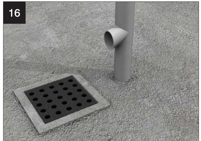
Ensure pitch is correct and structure is square. Fill holes around posts with appropriate concrete mix.
