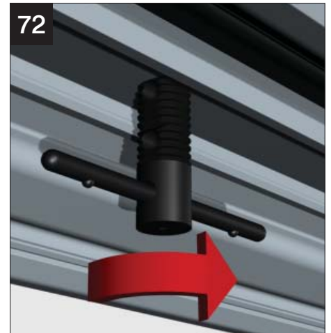
72 Twist through 90° to locate the T bolt into the ridge capping.
