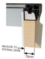
The minimum height of the kerb must be 150mm at it's lowest point. The kerb must have a pitch of  $4^{\circ}$ .
