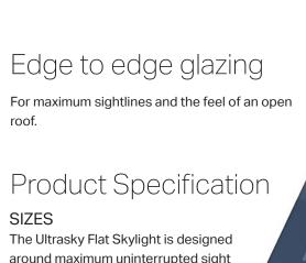
The Ultrasky Flat Skylight is designed around maximum uninterrupted sight lines and is available in a number of square or rectangular sizes ranging from 600mm x 600mm and going up to 2500mm in length (dependent on dimensions, see price list).
