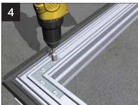
4 Fasten both fixings in both cleats on every corner
