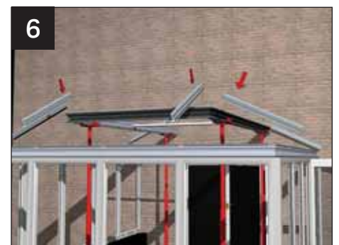
6 Now the Lantern eaves beam is assembled into a one piece structure, temporarily support it. Attach the glazing bars according to the component location plan. Tighten the bars, at the pagoda beam end first and then at the main eaves beam second.
