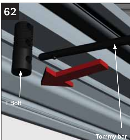
62 From the inside of the conservatory insert the snap off tommy bar into the T bolt
