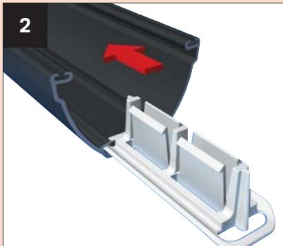
This stage should have been prepped in the factory. If not take the aluminium top caps and lay them onto a protected surface. Slide clips into each bar - position down from ridge / eaves at a max centre of 100mm and then at 500 centres (max) inbetween.
