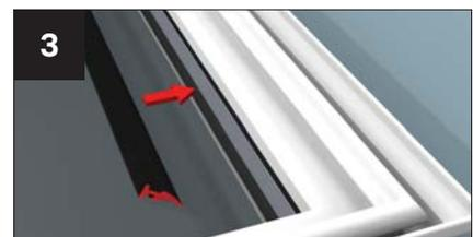
Now, invert the vent 'lid' (protecting the painted finish). Fit the wedge gasket, starting next to the manual vent bracket.
