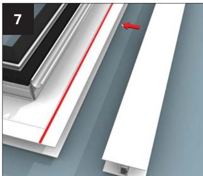
Now is the time to glaze the vent body into the roof. The vent is glazed in using two H sections at top and bottom. Prepare the upper H section using appropriate sealant in the four positions shown. See inset (step 6) to determine correct way round for 'H' section.
