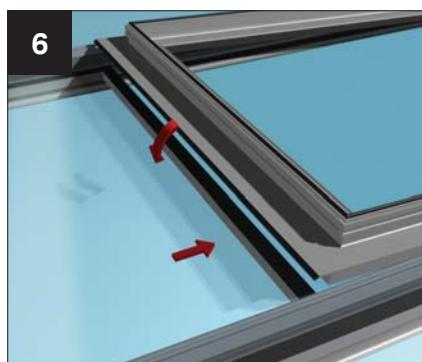
Lift the lower mainframe leg and offer into position the lower double glazed unit. Press down the mainframe firmly into position.
