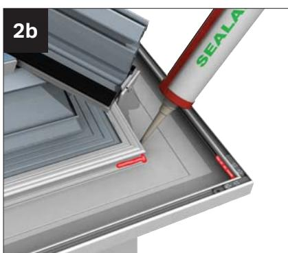
Silicone seal front and back edge of lower Cornice sections (be generous). Similarly butter 'DAM' sealer - position within 50mm of any stop end or outlet.
