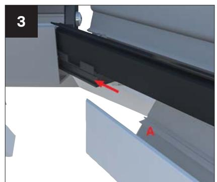
Position top of hips into ridge end ensuring they are butt up against it. Locate on the lip as shown above.
