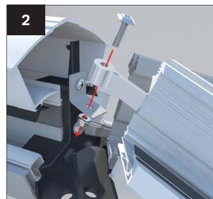
Depending upon the roof size and options requested, fit hub end transom bar and / or side transom bars. If specified on the job, remove nuts from bolts in transom position and fit transom bar over bolts. Re fit nuts and hand tighten. Check that ridge is level and fully tighten nuts on all bars.
