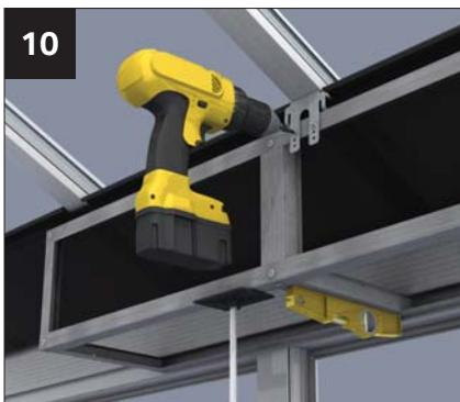
Attach L-Shaped frame using one of the three positions on the bracket, use 4 x 13 self-drill screws provided.
