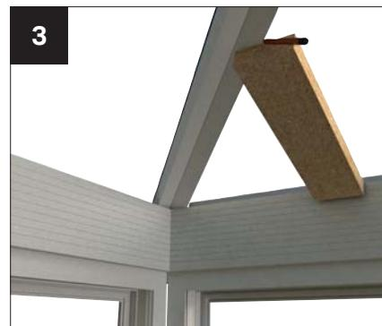
Use the location plan again for the hip positions. There will be a left and right. Mark these positions and then line up bracket and attach as before.
