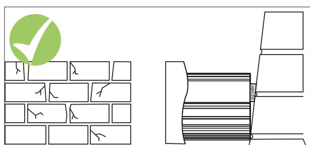
Check the condition of the host wall as this may affect the quality of the final installation. Check the host wall is plumb - any running in/or out should have been accounted for by the surveyor. If not, the ridge and starter bars may require packing out with aluminium shims. Correct alignment in this area is critical to a successful installation - Plumb frames/level ridge.
