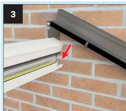
Fit the pre formed soaker trim to each starter bar, tighten the bars at the ridge and then at the eaves. Ensure the bar caps have been fitted.
