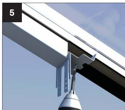
Take the transom bracket (CHA001) and attach using two 4.2 X19mm self-drill pan head screws (supplied). The back edge of the bracket should butt up to the under cladding.
