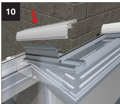
Knock down the glazing bar top cap so it finished flush with the bottom of the bar.
