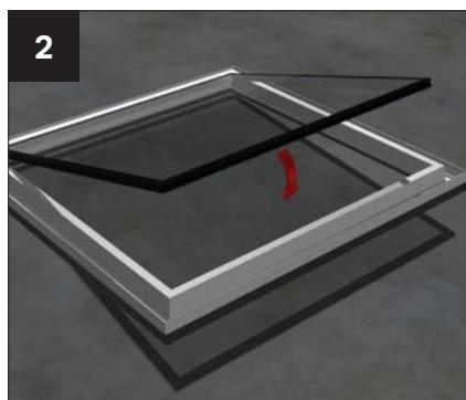
Remove all handling tape around the perimeter of the unit. When inserting the glazing ensure it is the correct way round and the external face is face down onto the continuous bead of sealant.
