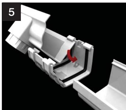
Next, build on the ground the gutter runs, by rolling items like a stopend under the back edge of a gutter jointer. Push up to the insertion line. DO NOT silicone seal, this would prevent natural expansion contraction.
