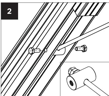
Attach the threaded bar through the barrel and then fit washer and two M10 nuts. Next insert the barrel assembly into the slot in the underside of the glazing bar and secure with a further two M10 nuts.
