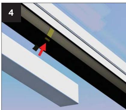
Locate the transom aluminium undercladdings on the bar, ensure they are tight up against the ridge.
