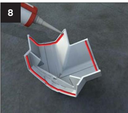
Apply generous beads of sealant to the underside of the external cover.
