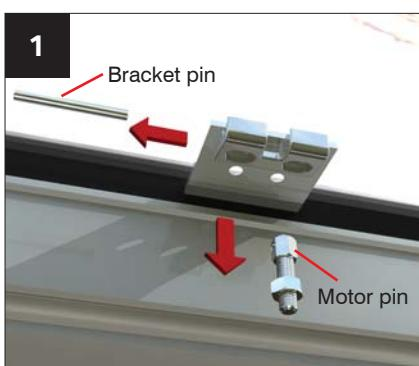
Pull out bracket pin to allow the vent motor pin to drop free.
