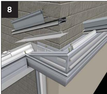
Place the short lengths of furring top cap and modified starter bar on to the two bolts. Please note that the bolts should be staggered, one each side of the bar.
