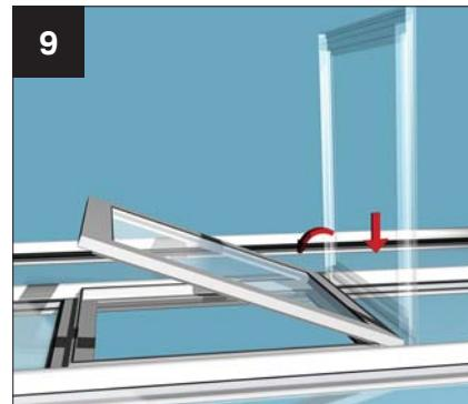
When the sealant on the mainframe has cured, re-fit the outer sash by holding vertically and re-engage on to the 'S' shaped hinge, before lowering into position. Refer to vent installation guide for further information about attaching the opening mechanism etc.
