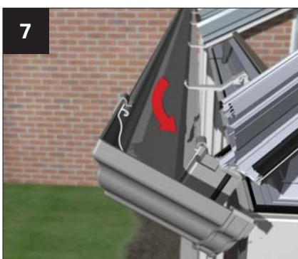
Locate the back edge of each section of gutter into the slot in the gutter bracket.
