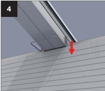
4 At the eaves hook a cloaking panel support clip over the fascia board at each transom.
