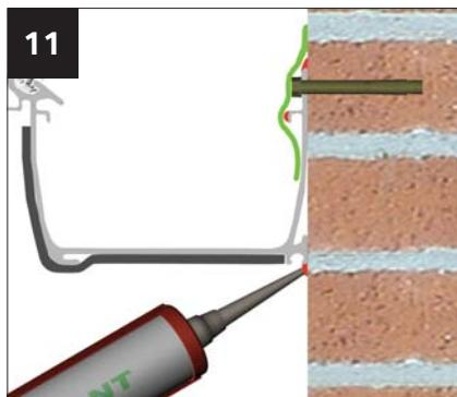
Seal the top and bottom edges of the aluminium box gutter, where it abuts the house wall.
