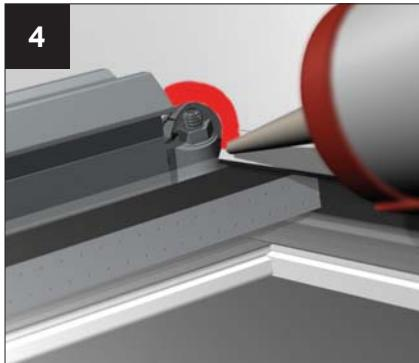
If using jack rafters, seal around the notched hip bar top cap ready to receive the jack rafter capping.
