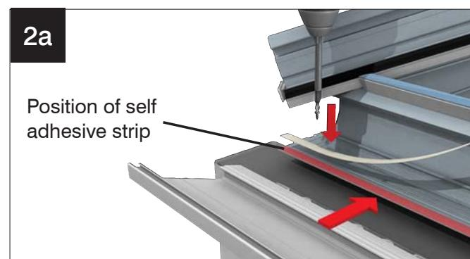
Attach self adhesive strip to 'toe' of eaves beam.
