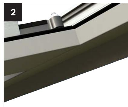
Now fit the jack rafters. The 2 part jack rafter kit is already fitted to the hip and jack rafter. Ease back the jack rafter undercladding. Each jack rafter kit is supplied with a number of washers. Trial fit the jack rafter and check that the glazing platforms are level. Adjust if necessary by adding or removing washers between the two part connecting kit, then tighten the nut. **NOTE: If aluminium internal claddings are being used, fit hip internal cladding prior to fitting jack rafters.**
