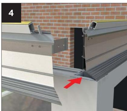
Place the next section of eaves beam into position, by slotting the corner cleat on the adjacent piece of eaves beam into the first piece.
