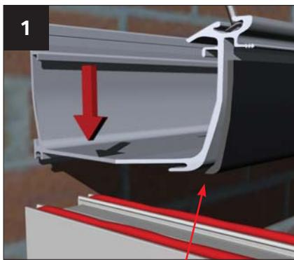
Box gutter foam to be cut back 70mm to enable the box gutter to sit flush on the frames.
