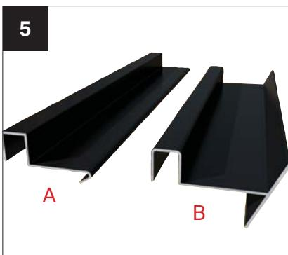
For PVCu internals, cloaking trim option A should be used. For aluminium internals, option B should be used.
