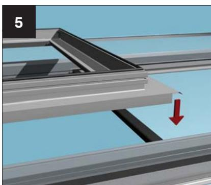
Carefully lower the frame into position on to the upper double glazed unit, making sure that any glazing tape has been removed from the edges of the sealed unit.
