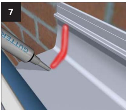
Now, from the bag in which the adaptor is supplied, take the special tube of sealant, Gutterbond. Apply a generous bead of it evenly across the mouth of the box gutter, 20mm back from the front edge.
