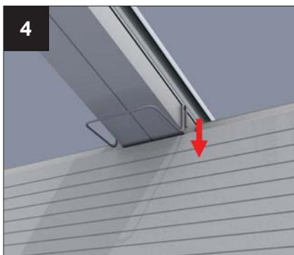
At the eaves hook a cloaking panel support clip over the fascia board at each transom.
