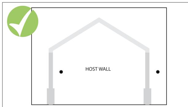
At this stage do not fix the frames down - pin only to the house wall (one fix per side) to allow the conservatory to 'float'.
