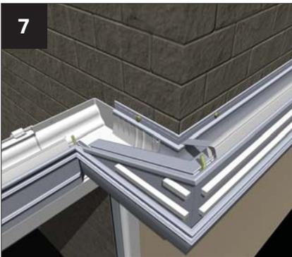
Following steps for the installation of box gutters on pages 21-22, check that the roofing bolts are in position (i.e top and bottom of the slope)
