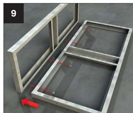
Assemble matching vertical and horizontal frames using the pre punched holes. \*See location plan for ladder layouts\*
