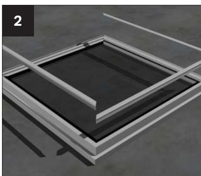
Re-fit the 'L' shaped serrated glazing beads to the opening sash. A small block of timber is useful to carefully knock in the beads.
