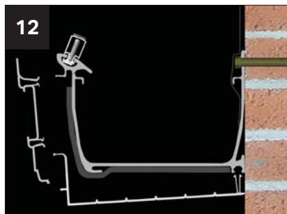
Before lifting into position, assemble the fascia board and undercladding. Offer up the undercladding rear legs, and knock up into position.
