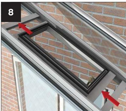
Apply bead of appropriate sealant to top edge of vent body and then slide vent body into upper H section. Repeat process for lower glazing panel. H section and insert into trailing edge of vent body. Ensure glazing/vent body are central between the two glazing bars.
