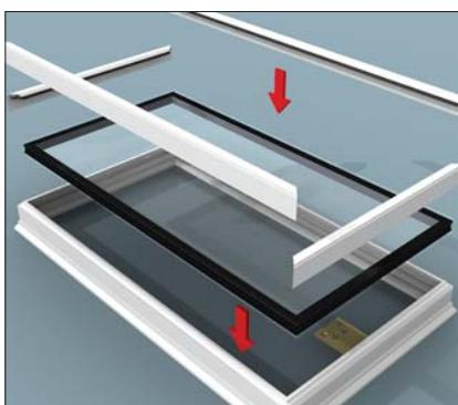
Remove vent 'lid' from the box and lay the correct way up on a protective clean surface. It may be easier to remove the winder mechanism. (See step 2a). Now fit glazing panel into place. Take the top and bottom un-mitred beads, run a bead of the appropriate sealant along both ends of the bead and clip into place. Now fit the mitre cut beads in the same manner.
