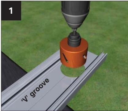
1 Decide the position of the gutter outlet by lining the extrusion 'v' groove up with the centre of the hole for the down pipe. Using a 73mm dia hole saw, cut the hole for the down pipe in the lower section.
