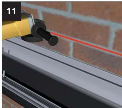
Mark out and grind a channel in the masonry for the flashing – blow out any dust in the channel.
