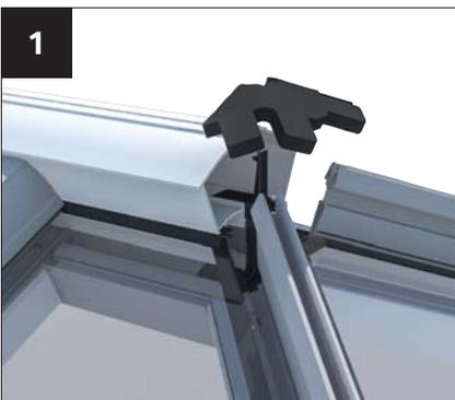
**ENSURE THE GLASS IS CLEAN AND DRY BEFORE FITTING.** Peel back protective film from weathering shield and position (adhesive face down) on glass, locating around the ridge and the hip bars. Press down firmly.
