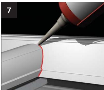
Seal around the joint on the jack rafter capping when complete.
