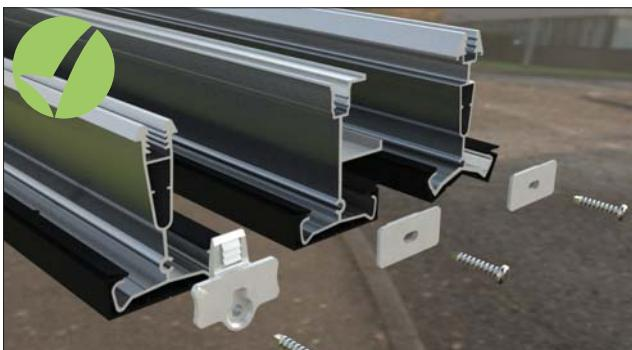
Attach the glazing bar end cap fixing blocks - as access restrictions (box gutter situations) may prevent easy attachment later. NOTE: These are attached to the end caps when despatched from the factory.
