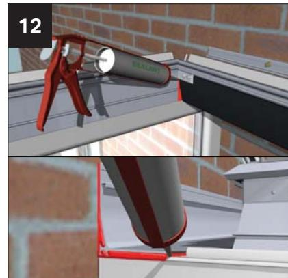
Now seal the internal joint between the eaves beam and box gutter and back point the leading edge of the box gutter where it sits on the side frames.
