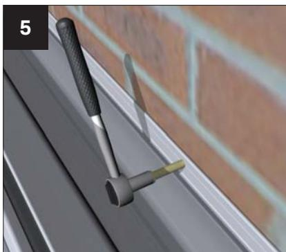
Offer the box gutter into position and insert the anchor fixings that are appropriate for the substrate and tighten up.
