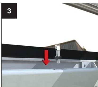
Screw motor pin into the top edge of the motor – adjust its height to fit with lid bracket.
