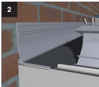
Place eaves beam section – with undergutter trim attached – onto the side frames. Seal the joint between the eaves beam and box gutter.
