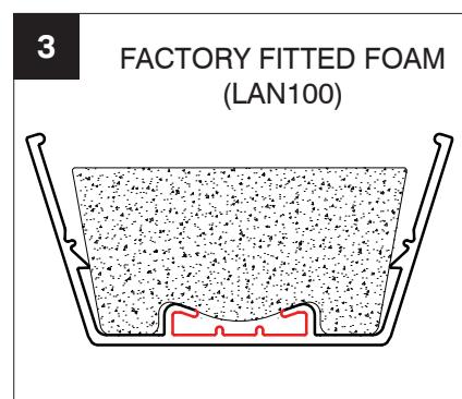
Ensure the foam does not interfere with the clips by pinching it towards the centre of the bar.
