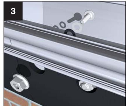
Drill 6.5mm holes through the box gutter and sleeve (at positions shown, ensuring both halves of the box gutter are flush together) and fix using the bolts, nuts and washers provided and in the order shown. Trim any excess off the bolt head before fitting the internal cladding as it may foul.
