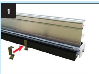
Attach spring clips (LAN014) to side of glazing bar - to each side of bar - 50mm from top of transom bar - 100 mm from eaves (both hip and transom). Push the leg in under the gasket and spring around the underside as shown. Ensure the clips are fully pushed on.
