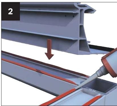
Apply a continuous bead of appropriate sealant to the front and inner legs of the window frames. Lift insulated box gutter into position – ensure it has adequate support whilst fitting.
