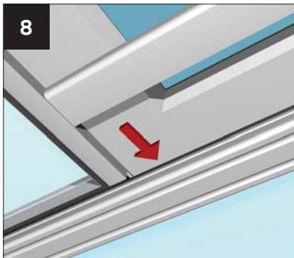
Down each side of the roof vent mainframe an 8mm thick PVCu architrave type packer is provided to suit the glazing thickness. Position as shown above.
