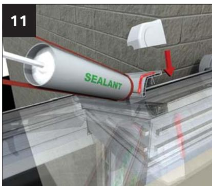
Two end caps are provided, one left hand and one right hand. Cut the appropriate end cap across its width (right hand shown) so that it fits snugly to the face of the glass, remove it and then using the correct sealant, refit.
