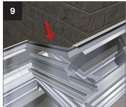
Lift the `L` shaped sealed unit into position and carefully position. Your office may have not ordered an `L` shaped unit but may have split the unit into two, use a muntin bar to joint them (see page 12).
