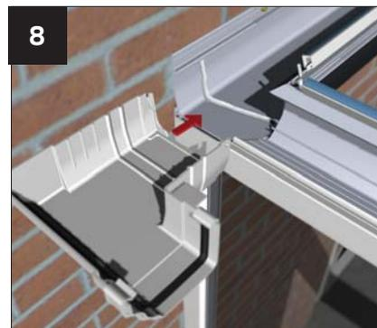
Slide the adaptor into the aluminium box gutter, raising up its front edge to utilise the unique `snow plough` effect. This spreads the Gutterbond evenly under the adaptor. Push the adaptor firmly up to its end stop, so that it will line through with the Classic gutter attached to the eaves beam.
