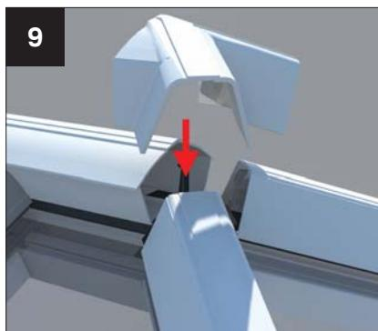
Press firmly down on the ridge end top cap until it clicks into position on the ridge end.
