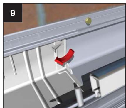
With the adaptor tight to the end stop, turn the toggles upwards to firmly press the adaptor into the Gutterbond.
