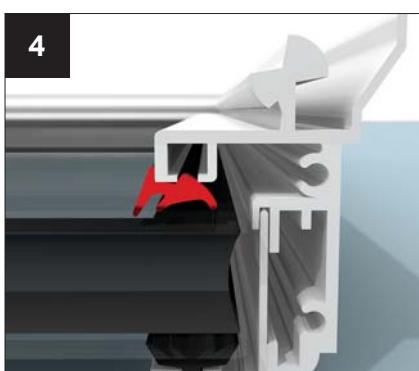
Insert gasket under vent under aluminium lip and work round the lid, cutting and notching in each corner and up to the vent bracket.
