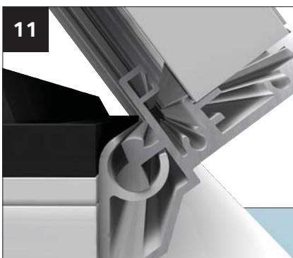
Lid knuckle will only engage with vent body hinge when lid is greater than 50 degrees. Once engaged, close lid.
