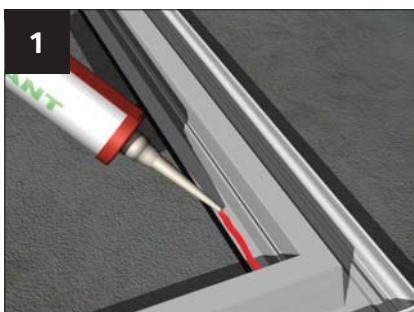
Remove the opening vent sash from the vent mainframe and lay the opening sash upside down on a flat surface. (Protect the surface to prevent damage to the sash). Run a continuous bead of appropriate sealant immediately behind the black co-extruded gasket, taking care to ensure a continuous run around the perimeter of the opening sash.
