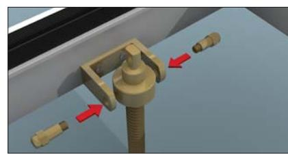
Remove the winder mechanism if pre-fitted – pull the spring loaded clip to release.
