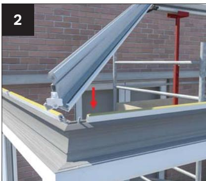
If not already attached, attach the glazing bar end cap fixing blocks - as access restrictions may prevent easy fixing later.
