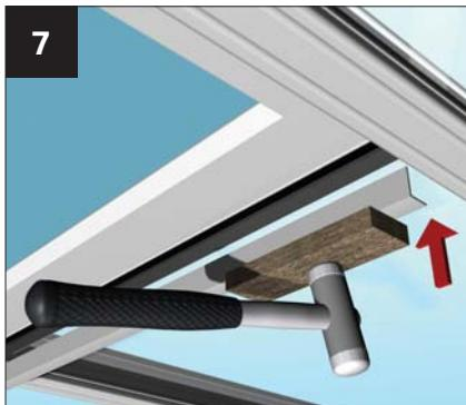
From inside, knock in the 'L' shaped serated glazing beads to the top and bottom edges of the mainframe.
