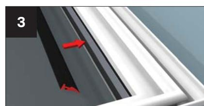
Now, invert the vent 'lid' (protecting the painted finish). Fit the wedge gasket, starting next to the manual vent bracket.
