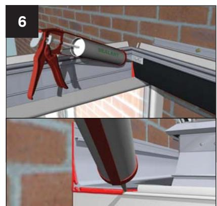
Now seal the internal joint between the eaves beam and box gutter and back point the leading edge of the box gutter where it sits on the side frames. Knife off a small section of the undergutter trim in preparation for the insertion of the adaptor.
