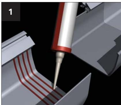
Thoroughly clean the mating parts using wire wool. Surfaces must be clean and grease free. Apply a generous bead of low modulus neutral cure to the pre-fixed internal sleeve along the entire face of the sleeve.
