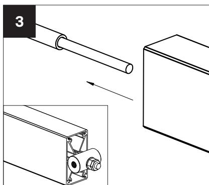
Now insert the PVCU tube (this acts as a damper) over the threaded bar and secure in place with double sided tape or silicone. Now insert the box section beam over the threaded bar/tube assembly.
