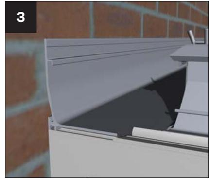
Place eaves beam section – onto the side beam and box gutter.
