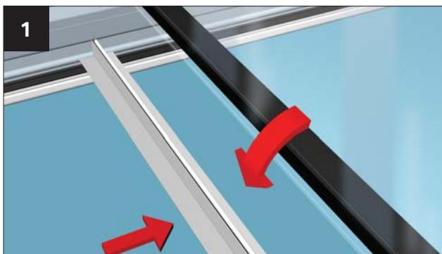
IF YOUR SEALED UNITS HAVE BEEN SUPPLIED WITH TAPED EDGES, ALWAYS REMOVE THE TAPE PRIOR TO INSTALLATION. Take the muntin bar profile (top and bottom section) that matches its corresponding sealed unit. Take the lower section and allow it to span between the two adjacent glazing bars. Lower into position the up slope sealed unit. NOTE: MUNTIN SHOULD BE SAME WIDTH AS UNIT.
