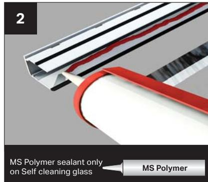
2 Seal underside of top face of glazing end profile as shown (PVCu version of end profile is shown - if aluminium glazing bar top caps, this end profile is also aluminium).
