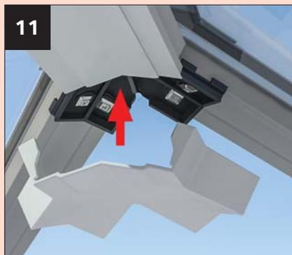
11 Fit the internal plastic cover if supplied by pushing up into position over the ridge and ridge end.
