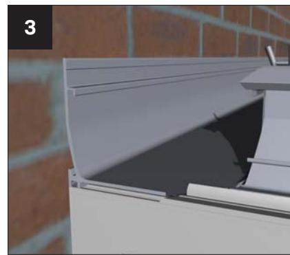
Place eaves beam section – onto the side frames. Seal the joint between the eaves beam and box gutter.
