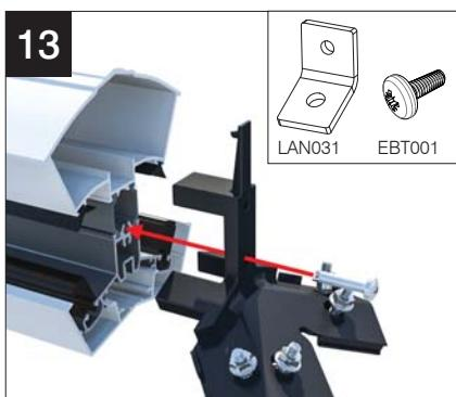
LANRF001 is supplied pre-installed into the ridge. Remove and fix radius end (LAN032BL) then replace the screw. If using 3 bar attach LAN031 using EBT001. (M5x12 P021 pan screw).
