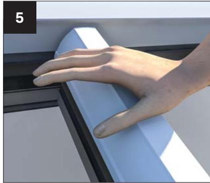
5 Using the heel of your hand, push down on the top cap to engage the clips, working from ridge to eaves. Ensure the rubber gaskets are full compressed for a watertight seal. NOTE: on longer bars it may be necessary to use a soft mallet and timber block
