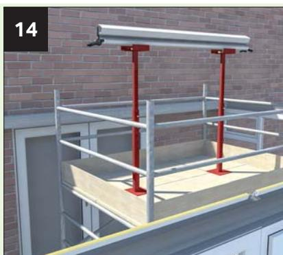
Prop ridge in position using suitable supports, centralising between eaves beam sections. (When the ridge features aluminium painted internal finish it will need to be protected whilst supporting).
