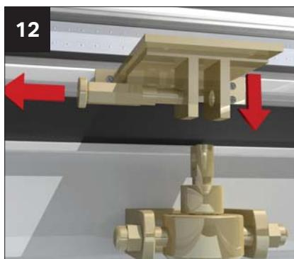
Now is the time to fit the spindle ( if manually controlled). Remove spring pin if not already done. Attach spindle to lid. Now unscrew bolts in vent body, unwind spindle to correct height to align with bracket. Screw in bolts to secure spindle in position and re-attach spring pin.
