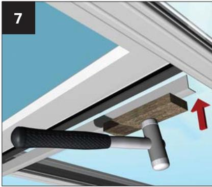
From inside, knock in the 'L' shaped serrated glazing beads to the top and bottom edges of the mainframe.
