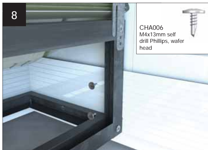
Fix the vertical frame into the fascia board using 2x CHA006 (M4 x 13mm) self drill Phillips, wafer head screws (supplied).
