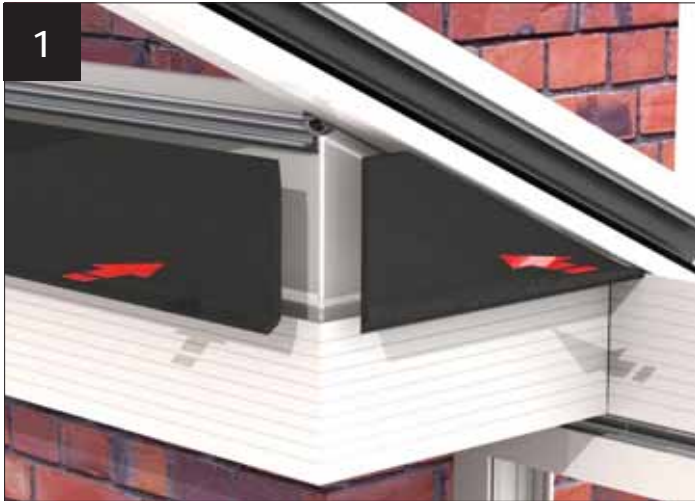
1 If not already fitted, attach boxgutter insulation foam to the upper section of box gutter.
