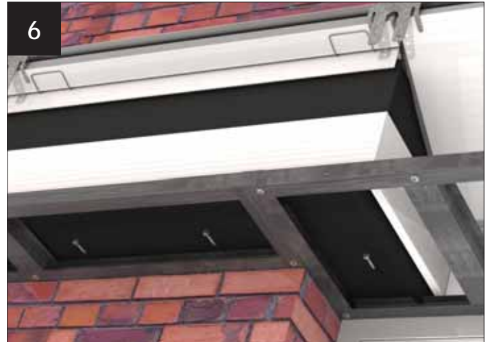
6 Fit back horizontal frame using CHA008 (bag of 25) as per standard installation.
