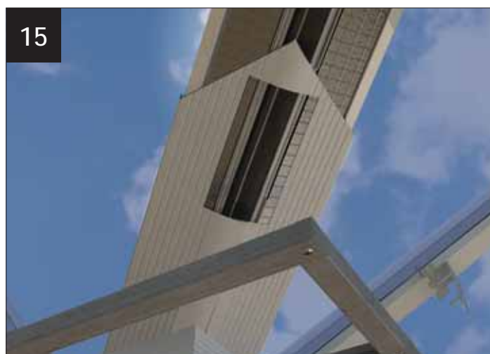
15 Fit the valley plate CHA016 (refer to steps 1-5, valley standard classic).
