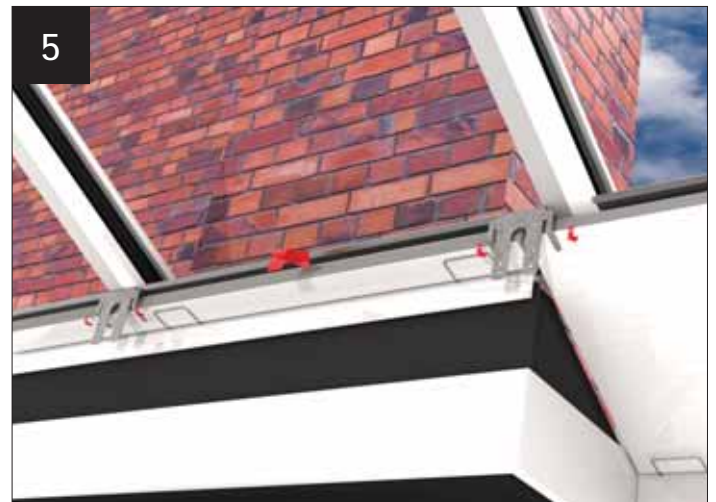
5 Fit the polycarbonate modesty panels and bend over bracket legs to secure.
