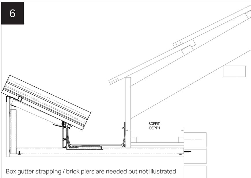
Box gutter strapping / brick piers are needed but not illustrated
