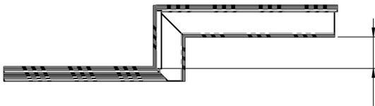
Plan View: Raised back box gutter
